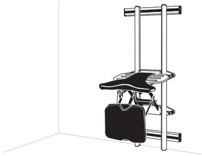
**The pivot configuration** can be used as a transfer aid to a stationary toilet. Without the kneeboard, the padded trunk board can pivot 180°. Installed near a standard toilet, a client can use the Support Station to assist in sit-to-stand from a wheelchair and rest their torso on the padded trunk board. Then, while moving the feet, a client can be pivoted to a position close to the toilet.
